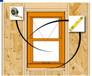
Place a level on the window sill to verify that the sill is level. Adjust the shims as needed to ensure a level condition. Check the head, sill and jambs with a level again to make sure the window is setting plumb, level, and square within the opening. Measure across the diagonals to determine if the window is square. Add shims around the entire window as needed to ensure a plumb, level, and square installation.
