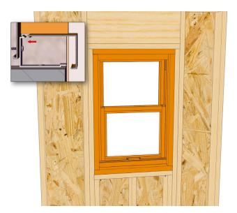
Insulate between the window frame and the rough opening using minimally expanding window and door spray foam or fiberglass insulation that is compliant with AAMA 812-04. Apply sealant continuously around entire perimeter of opening after foam or insulation is installed. Read and follow the manufacturers' recommendations for application and use. Measure and trim the snap covers to fit the opening, widths then heights. Install the snap trim covers to finish the interior.
